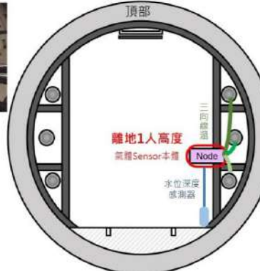
Real-time Underground Cable IoT Status Detection and Wireless Life Alarm
